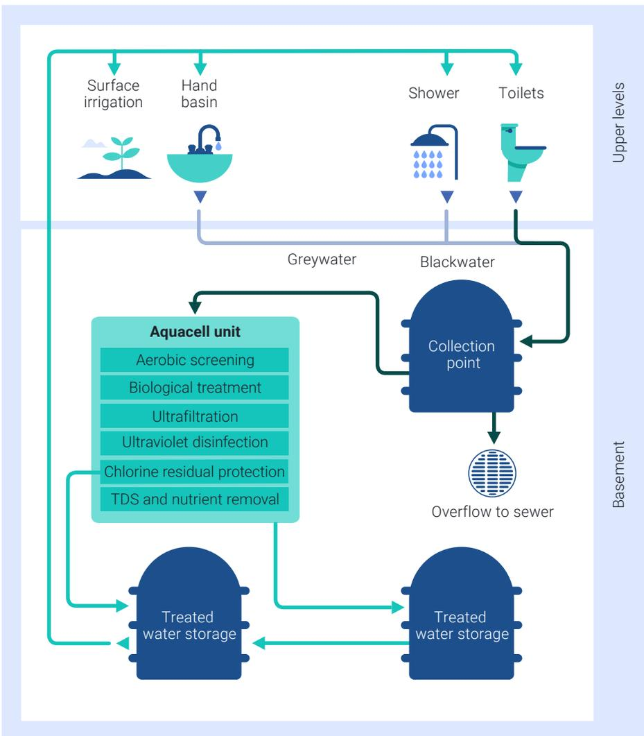
← The efficient blackwater treatment system collects used water from different parts of our operations before running it through several processes that make it safe for reuse.
